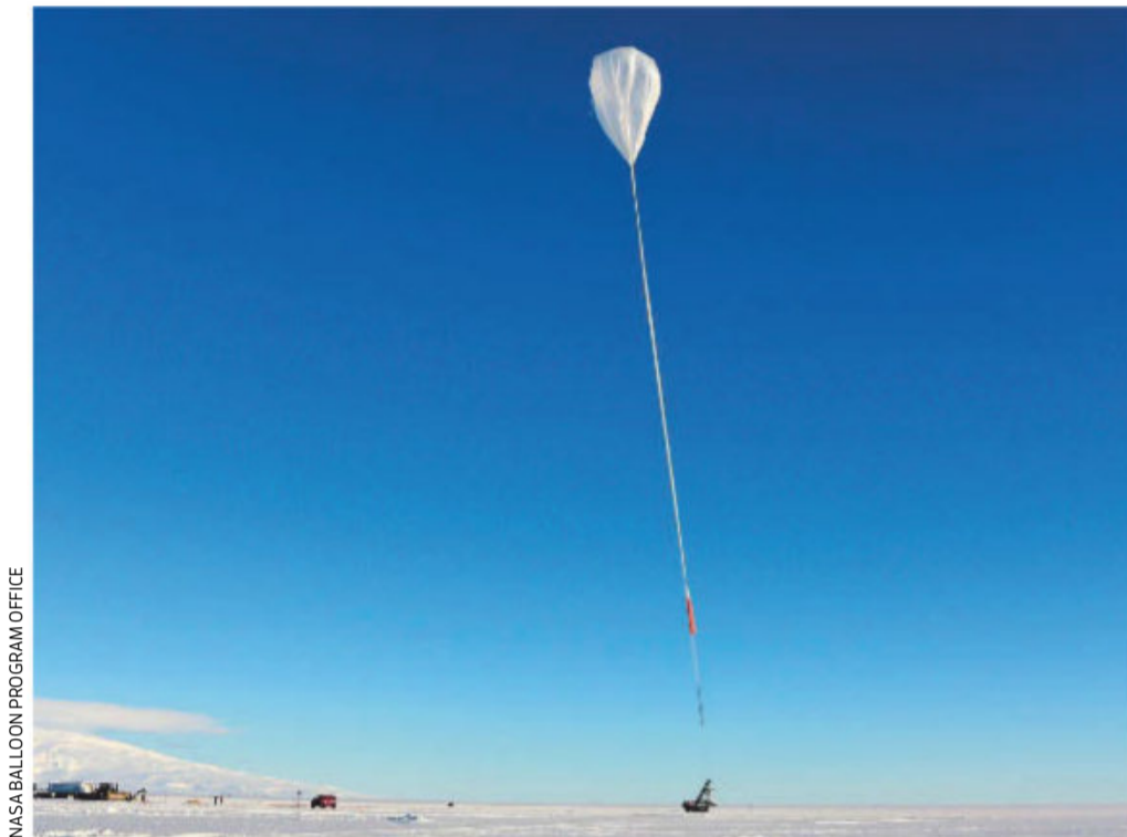
The balloon-mounted ANITA experiment surveys more than a million square kilometres of Antarctic ice for signals from cosmic rays
