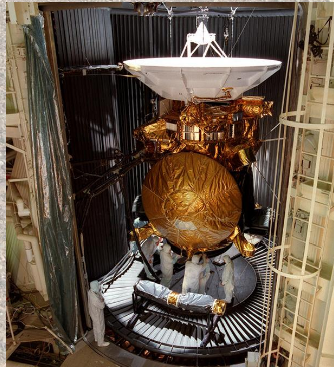
The Cassini-Huygens spacecraft during the Solar Thermal testing
