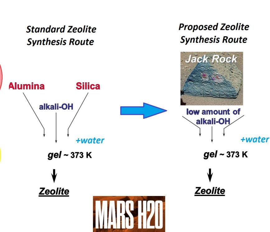
Zeolites are conventionally made from pure chemicals to obtain solutions of sodium silicate and sodium aluminate, which are mixed in appropriate proportions into form a homogeneous gel. Clay minerals have attracted a lot of attention to be used as a source of alumina and silica for production of zeolites.
