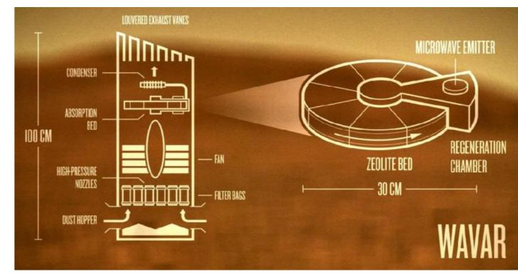
method. The produced zeolites can be used in WAVAR to produce more water which serves for In Situ Resource Utilization (ISRU).
