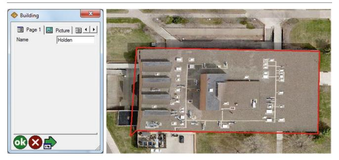
**Result**: The Holden building is captured and it is shown in red. The boundary of the building is not exactly delineated due to GPS accuracy. This offset will be corrected later on in the office using ArcMap.
