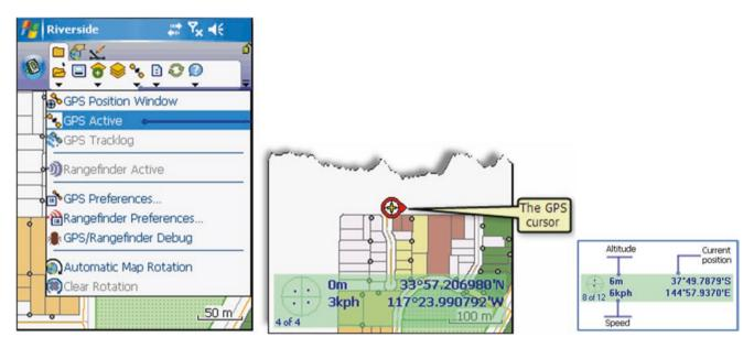
**Result**: The GPS cursor is displayed as a red circle with a cross inside it, and a small tail. The location (latitude–longitude), the altitude, and speed are also displayed.
